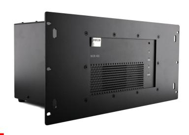
The MCM-400 HDF serves as input processor on Barco's Galaxy/HDQ 4K series projectors allowing geometry correction, color correction, brightness monitoring and electronic blending. By using a real-time on-screen user interface, the MCM-400 HDF helps achieve the performance known from Barco's higher end 4K simulation projectors. In this way, this box enables several multi-channel configurations with multiple 4K projectors.
